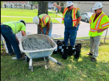
Concrete Strength Testing
